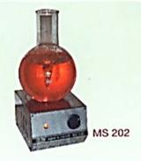
These equipments are intended for stirring solutions of low viscosity in open or closed vessels. Stirring is accomplished by a magnetized teflor coated paddle to be placed in the container. Each apparatus of this group can be operated on a bench, a stand or a laboratory scaffold as well. The intensity of stirring, depending on requirements, can be adjusted with the thyristorised voltage controller incorporated which also ensures step less adjustments from very low to the maximum agitation.
